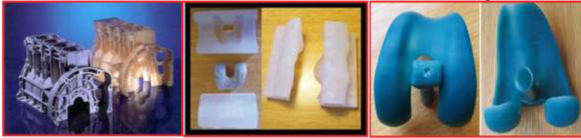
Fig. 43 Complex pattern (RP). Fig. 44 Silicon mold. Fig. 45 Prototype of wax pattern.
