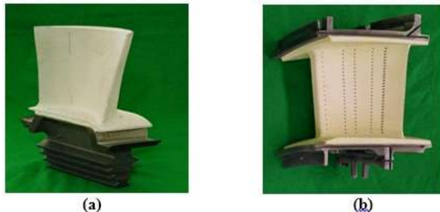
Fig. 30 Turbine (a) Blades and (b) Nozzle guide vanes show the internal cooling channels.
